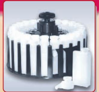
The reagent plate can hold up to 24 bottles ranging in volume from 35 ml to 6 ml. The entire plate (including the reagents) can be easily removed from the instrument for refrigerated storage.
