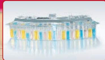
Thanks to the automatic washing of the six 20 - cuvette racks, there is no need for the operator to intervene during routine running.
