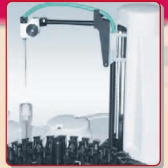
The single sampling arm connected to an integrated diluter module (no consumable or glass parts) guarantees extremely high accuracy and minimum risk of contamination thanks to the programmable automatic washing of the sampling probe at every analysis cycle. The instrument's level sensor prevents sampling errors and makes it possible for the operator to have constant updating regarding reagent consumption.
