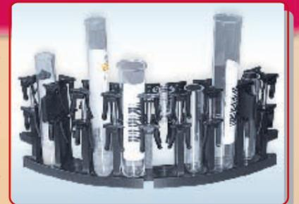
With its four individually removable racks, new samples to be tested can be added or STAT exams immediately carried out without interrupting the readings already programmed and underway. Either primary tubes or sample cups (for minimum quantities of serum) can be used.
